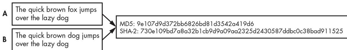
Figure 5-8: In a hash collision, two distinct messages produce the same hash.
