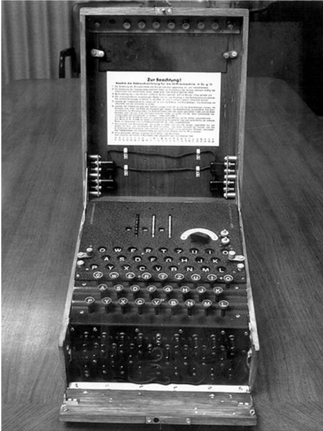
Figure 5-4: An Enigma machine
